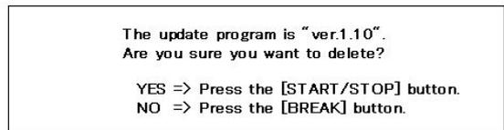
4. To delete the upgrade data, release the [START/STOP] button and then press it once again.
