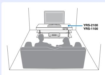
This unit uses sound beams to create surround effects (the arrows in the following diagrams indicate the images of paths of 5-channel sound beams). To achieve desired surround sound effects, install this unit where there are no objects such as furniture obstructing the path of sound beams.
