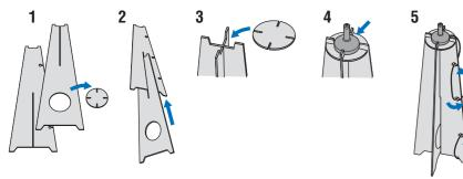
Use the supplied cardboard microphone stand or a tripod to place the IntelliBeam microphone at the same height as your ears would be when you are seated.
