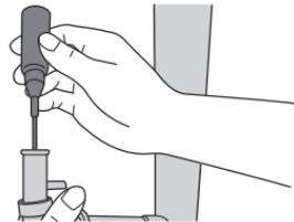
2. Remove the rotary valve cap and apply a small amount of rotor spindle oil to the center of the rotary valve and the area supporting the shaft.
