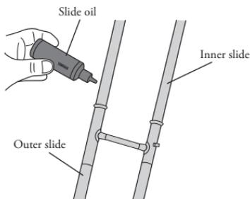
2. \* Only when applying a slide cream After applying a slide cream, use a water spray bottle to moisten the slide sufficiently.
