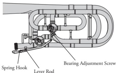
3. Carefully remove the 2nd valve section making sure the parts do not come in contact with the instrument.
