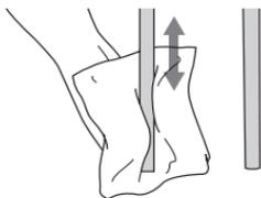
3. Wrap a cleaning rod with gauze so there is no bare metal exposed.
