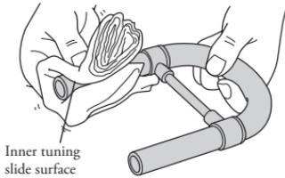
2. Wrap a cleaning rod with gauze and remove dirt from the interior of the inner and outer tuning slide.
