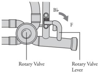
On trombones with double rotary valves, the levers can be used to change the pitch from B $\flat$ -F, B $\flat$ -G $\flat$ , B $\flat$ -D.
