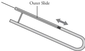
\* Use a cleaning rod wrapped with gauze to clean out the inside of the inner slide.
