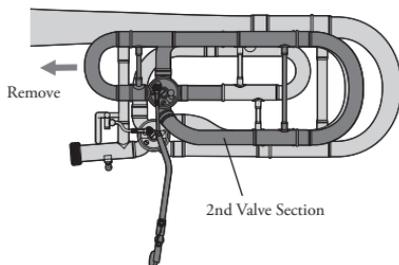
4. Attach the included F-valve slide to the instrument, paying attention to the insertion direction.
