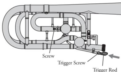
2. Hook the end of the spring onto the spring hook. Next, loosen the lever rod to remove.
