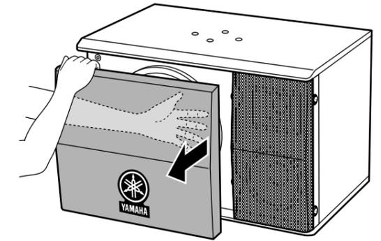
3. Remove the 4 screws that hold the metal speaker grille.
