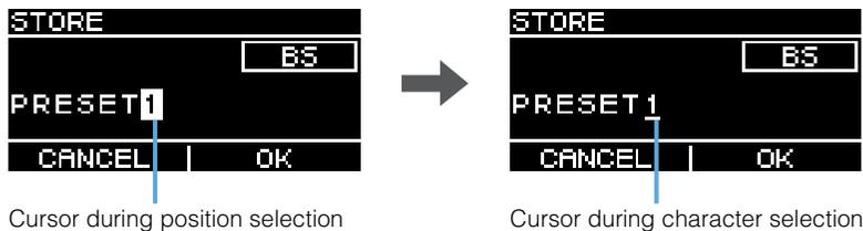
Turn the main knob to select the position to enter text, and then press the main knob to enter text input mode. When in text input mode, turn the main knob to select the character you wish to enter, and then press the main knob to enter the character.
