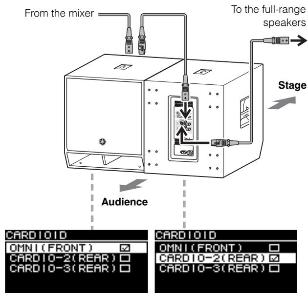
● **Screen when three subwoofers are placed side by side**
