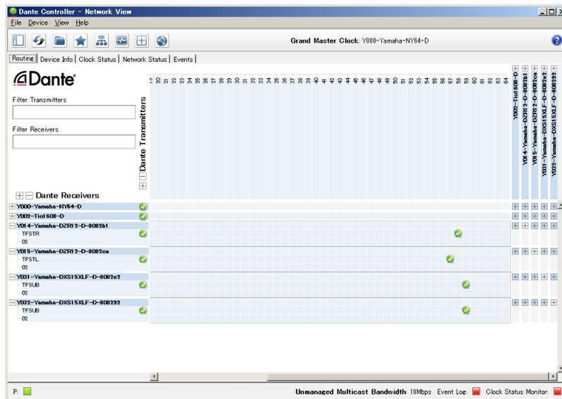
For more details, see the Dante Controller User's Manual. Also, for more information about the Dante channels assigned to the output signals from the transmitting devices (digital mixers, etc.), see the relevant manuals for the transmitting devices.
