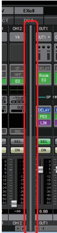
By dragging the scroll bar in the center of the screen to the left or right, you can change the proportion of input channel faders and output channel faders that are shown.
