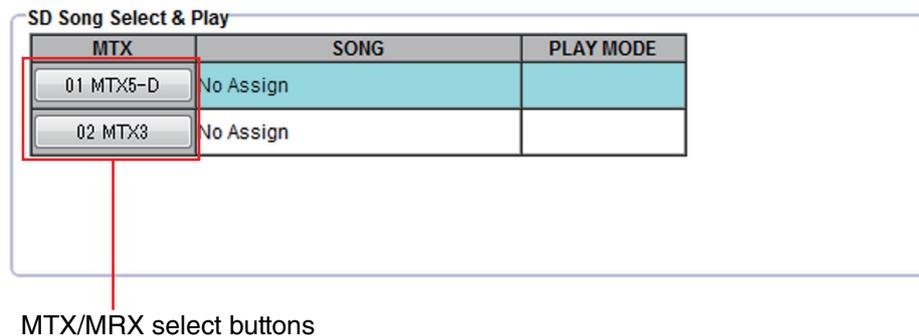
Here you can specify a file that will be played when the preset is recalled. Each MTX/MRX unit can play one file or play all files in the same folder in ascending alphabetical order. If four MTX/MRX units are connected via YDIF, up to four files can be played simultaneously.
