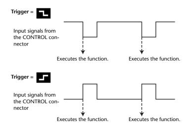
At this point, when the 02R96 receives the trigger signal at the CONTROL connector, the selected parameter changes.
