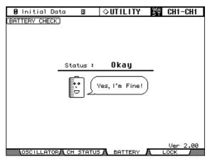
If the Status is "Okay," the battery is okay. If the Status is "Getting Low," ask your Yamaha dealer to replace the battery as soon as possible. Do not attempt to replace the battery yourself. Failure to replace a low battery may result in data loss.
