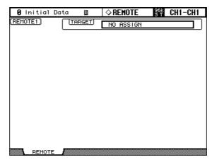
2 Use the cursor buttons to select the TARGET parameter, use the Parameter wheel or INC/DEC buttons to select USER ASSIGNABLE LAYER, then press [ENTER].
