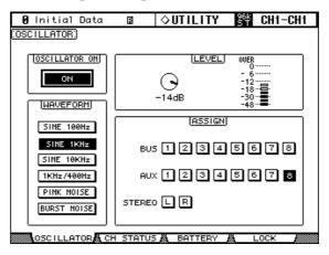
2 Use the cursor buttons to select the parameters, and use the Parameter wheel, INC/DEC button, or [ENTER] button to set them.
