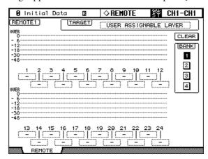
3 Use the cursor buttons to select parameter 1–24, use the Parameter wheel or INC/DEC buttons to select a channel you want to assign, then press [ENTER].
