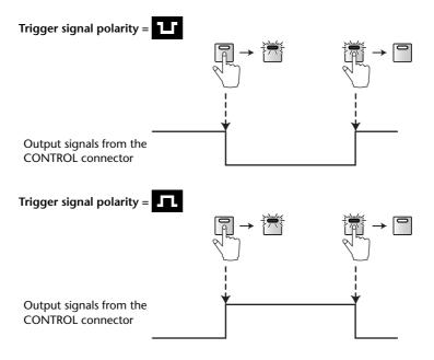
At this time, the trigger signal is output from the CONTROL connector when you operate the assigned parameters or controls.
