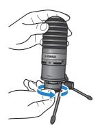
3 If necessary, adjust the angle of the microphone by loosening the knob while supporting the microphone, then retightening the knob.
