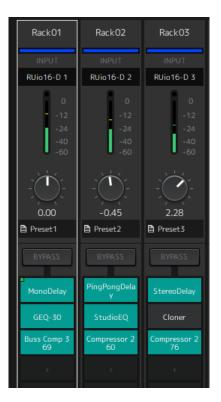
You can drag racks to reorder them within a bank. When doing so, channel assignments do not change. Each bank can contain a maximum of 16 racks, whether Mono or Stereo. If the maximum number is exceeded when you bring in a rack from a different bank, the last rack in the bank (the rack in the rightmost position) moves to the next bank. The same applies if the maximum number of 16 racks is exceeded when you unpair two racks.
