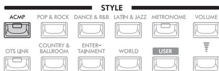
The Lower Keyboard is enabled for use as the chord section, and chords played in this section are automatically detected and used to generate fully automatic accompaniment with the selected Style. The Pedal Voice does not sound while the [ACMP] button is on.
