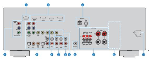
The area around the video/audio output jacks is marked in white on the actual product to prevent improper connections.
