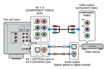
If you select the input source by pressing AV 1–2, the video/audio played back on the video device will be output from the unit.
