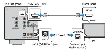
If you switch the input source of the unit to "AV 4" using the AV 4 or SCENE(TV) keys, the TV audio will be played back on the unit.
