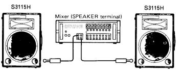
\* Connect the power amplifier's speaker output terminal and the speaker system's plug in the proper polarity. The polarity of the speaker-side plug is shown below.
